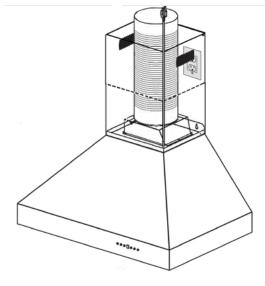
NOTE: Run the electrical cord up the chimney, outside of the ducting, and plug into a dedicated power outlet on the wall or in the attic. An outlet behind the chimney, to either the left or right, is ideal. Figure 5, left
