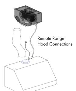
NOTE: The remote blower must be kept inside the home, such as the attic or crawl space. Never try to install a remote blower outside of the home.
