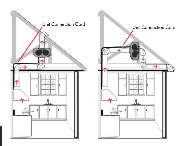
Single and dual-motor remote blowers are designed to reduce noise by installing them in a separate location inside the home, up to 20' away from the range hood.
