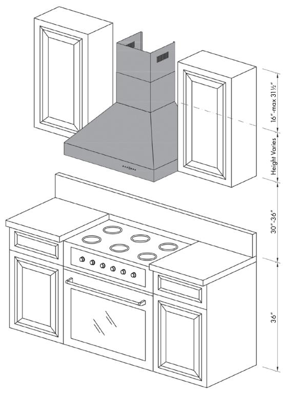
NOTE: The recommended height to install your hood is 30" minimum and 36" maximum above the range top or cook top. For outdoor range hood installation, the unit must be installed at a minimum of 36" and a maximum of 42" above the grill. These distances allow for maximum venting efficiency. The height of your chimney will vary depending on model of hood, as well as the height of your kitchen ceiling.
