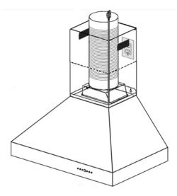
NOTE: Run the electrical cord up the chimney, outside of the ducting, and plug into a dedicated power outlet on the wall or in the attic. An outlet behind the chimney, to either the left or right, is ideal. Figure 6
