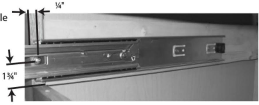
**Step 4.** Using the 5mm Allen wrench, and 10mm wrench, remove the board and front support from the friction slide units.
