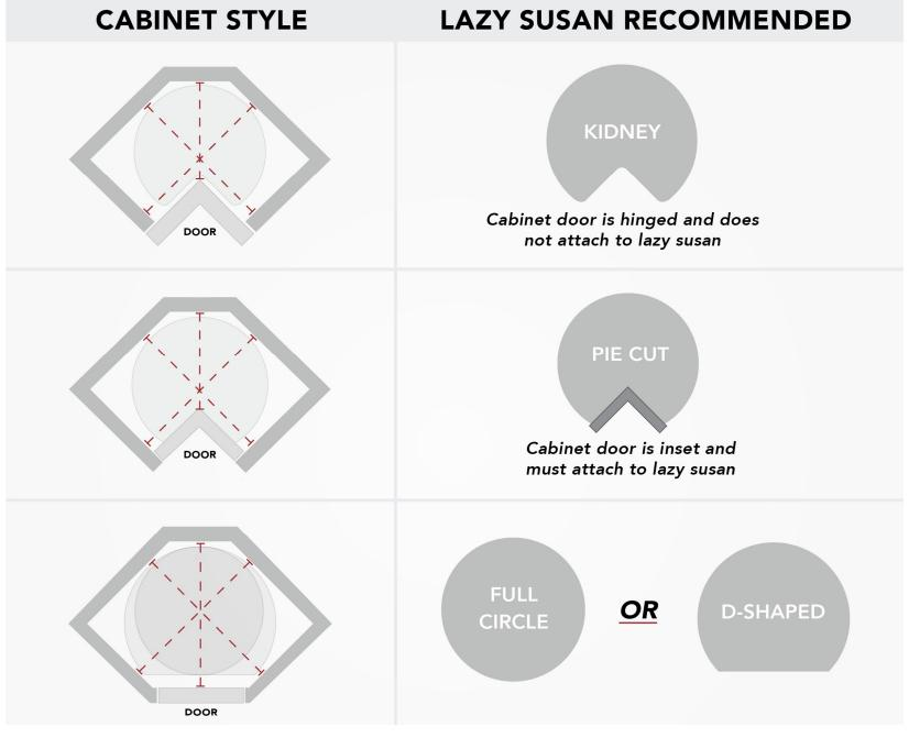
1 DETERMINE CABINET STYLE 2 MEASURE INTERIOR CABINET OPENING AS SHOWN ABOVE 3 COMPARE MEASUREMENTS TO THE AVAILABLE PRODUCT SIZES/DIMENSIONS TO VERIFY FIT
