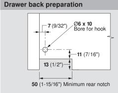
Drawers **must** have **6** holes drilled in the back panel to accept the hooks on the MOVENTO runners. Drawers must also be notched in the back, flush with the drawer sides and drawer bottom.
