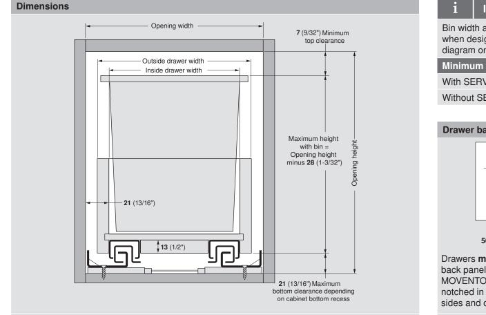
**NOTE:** Drawer side material thickness may vary. Accurate measurement of drawer side material thickness should be used when calculating outside drawer width using the table below. Inside drawer width **must** equal opening width minus **42** for MOVENTO to align and function optimally.
